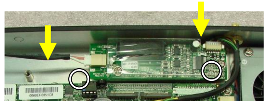
2. Disconnect the LCD cable to uncover the inverter board.
