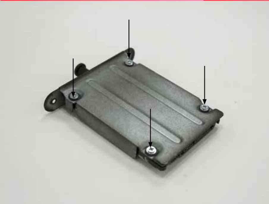
5. Remove the 4 screw on the back side of the storage device
