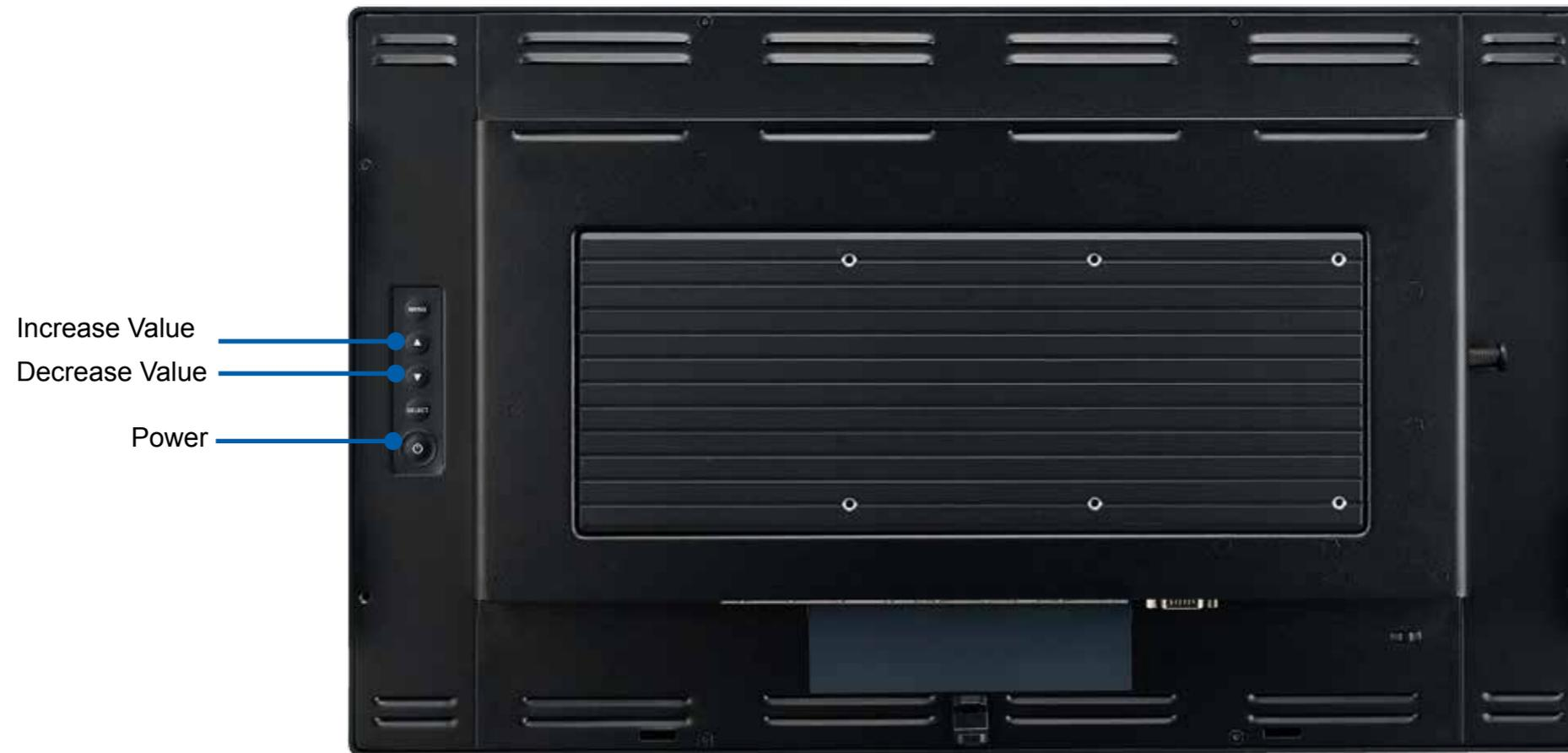
1. Press the "Power" button to on/off computer system
