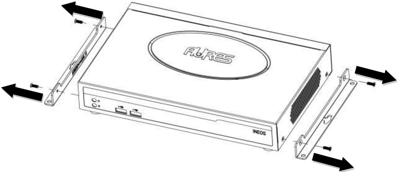
Likewise, you can assemble the box with mount brackets back by fastening the screws (x 4) by the side of box PC based on the direction.
