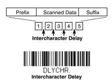
To remove this delay, scan the **Intercharacter Delay** bar code, then set the number of delays to 0. Scan the **Save** bar code using the **Programming Chart** inside the back cover of this manual.
