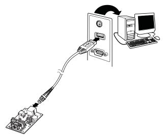
If using high-speed USB, connect the USB interface cable to side of the engine and to the USB port on the computer.
