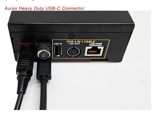
A custom 1.8-meter (6ft) cable has been designed for connecting the Aures POS HUB to Aures POS computers, including the Yuno II, Jazz, Jazz Pole, and Twist models. When using this cable, neither the I/O module nor the power supply adapter is needed for these computers, as the single USB-C cable suffices for all connections to the POS.
