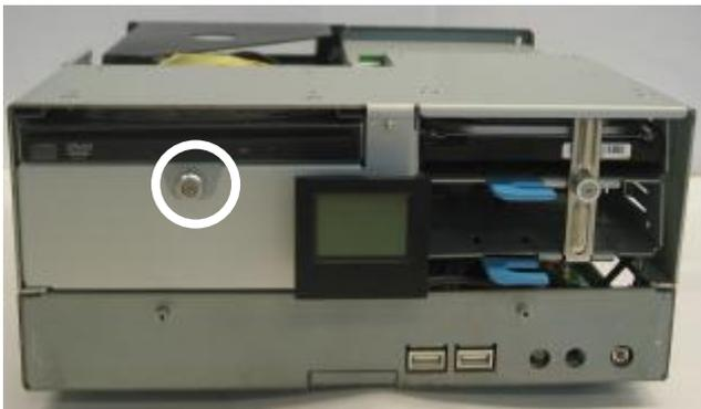
a. Loosen the thumb screw (1)
