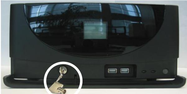
a. Open the front cover door and unlock it with the key.
