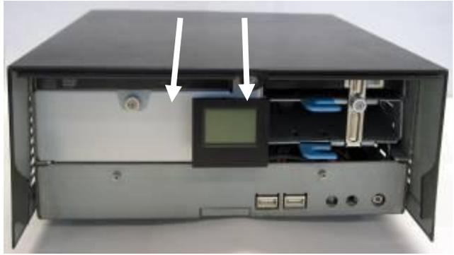
b. Slide the top cover towards the front and remove it from the system.
