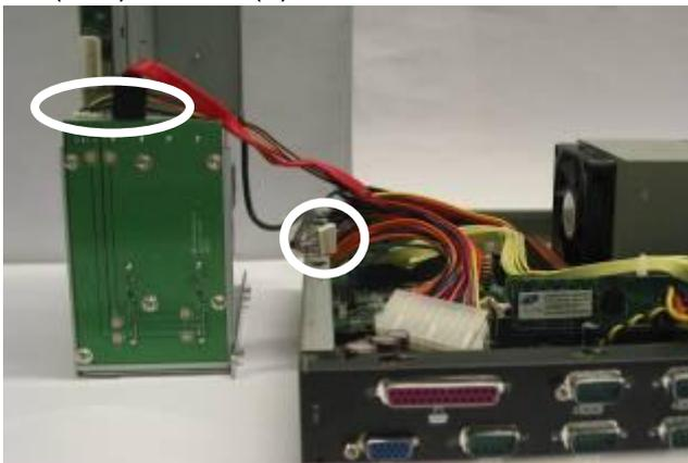
a. Disconnect the HDD power cable and the SATA cable from the HDD docking board. Disconnect the Hardware Status Display cable.
