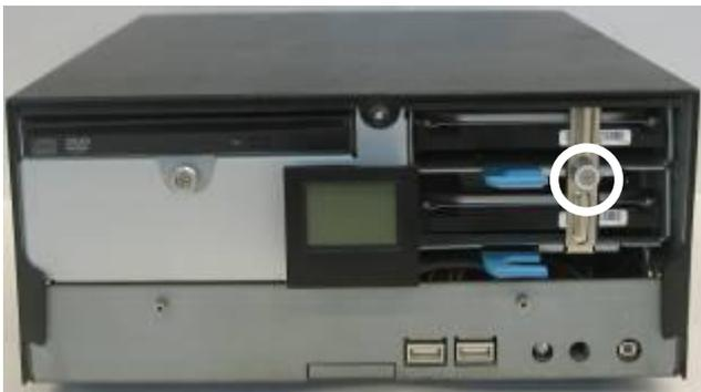
a. Loosen the thumb screw (1).
