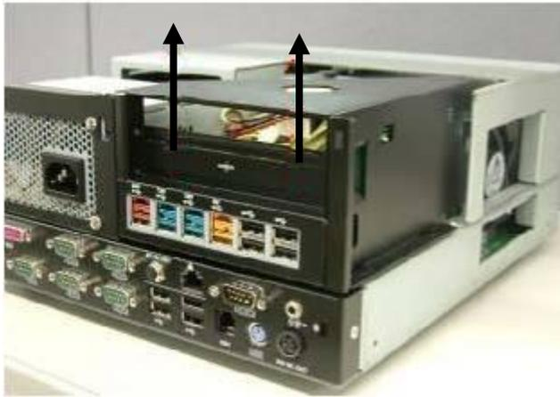
a. Remove the extension module by gently pulling it upwards taking care not to damage the connector.
