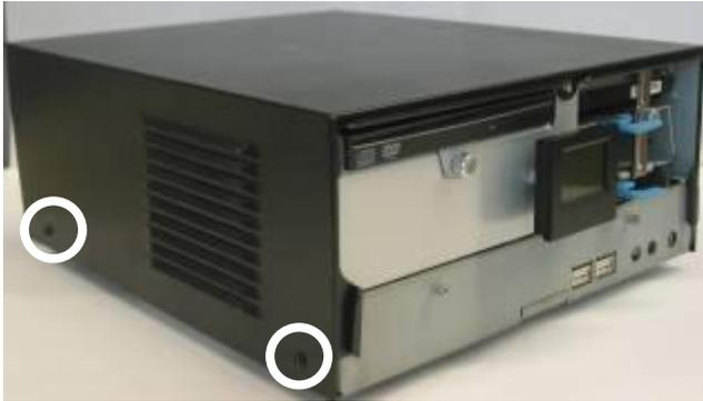
a. Remove the two screws on each side of the top cover
