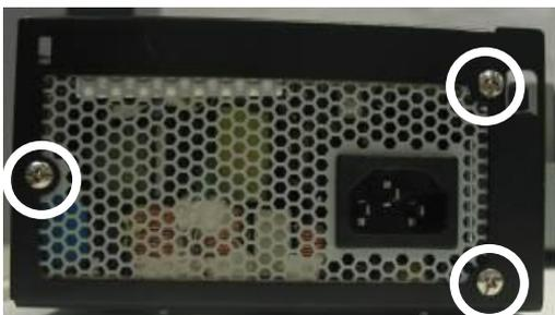
e. Remove the screws (3) to separate the power supply from the holder.
