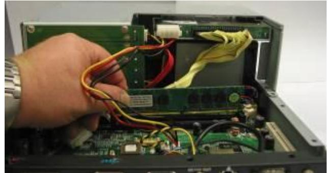
b. Remove the memory module from the slot.
