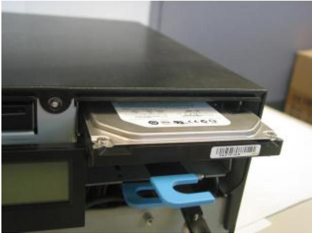
c. Pull on the blue tab to remove the HDD.
