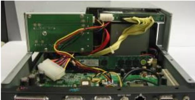
a. Use your finger to push the DIMM slot ejector clips into the down position.
