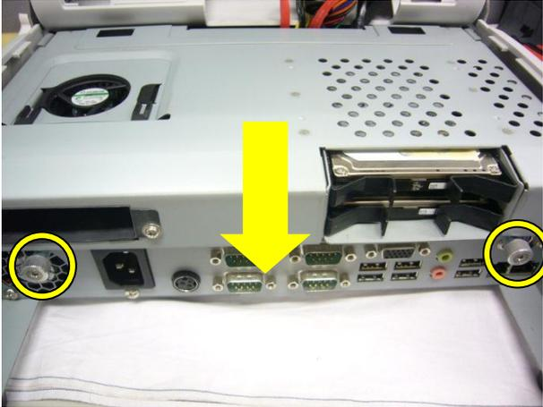
a. Loose the thumb screws (2), and slide the base cover bracket towards you to open up the system.
