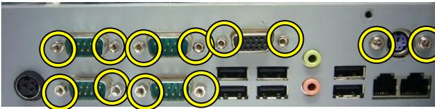
c. Remove the screws (12) securing the I/O panel.
