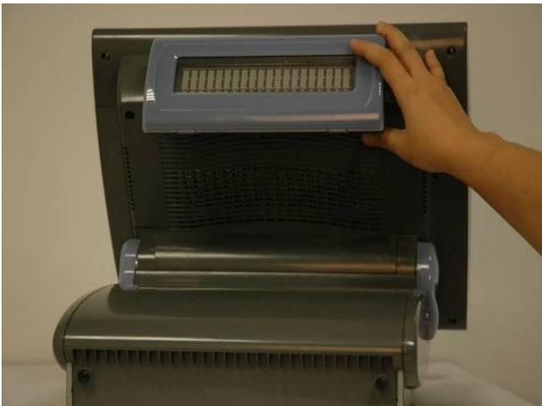
i. Slide the CPU ram door into position.
