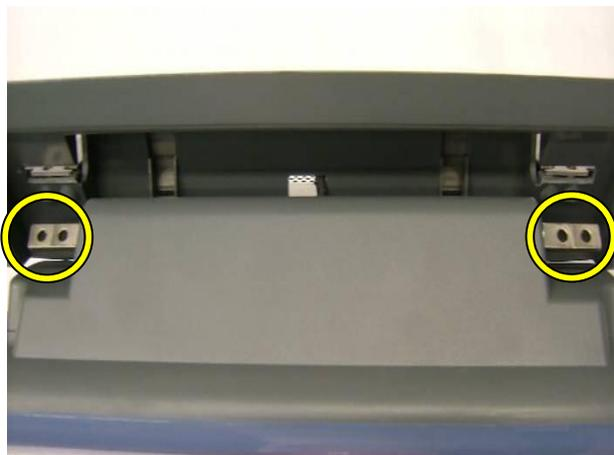
f. Click both sides of the VFD assembly into the position as shown in the picture.
