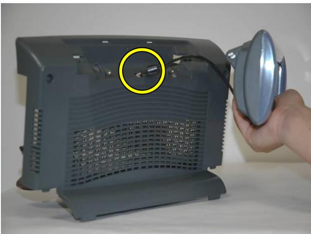
e. Pass the VFD cable through the hole as shown in the picture.
