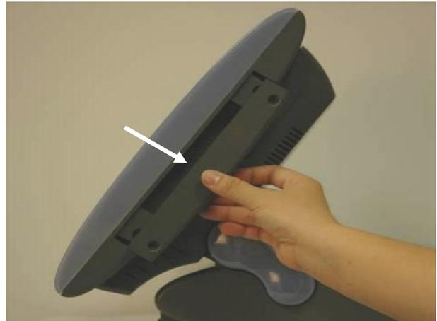
b. Slide the MSR dummy door out as shown in the picture.
