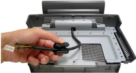
e. Install the ferrite core around the VGA cable and close it.
