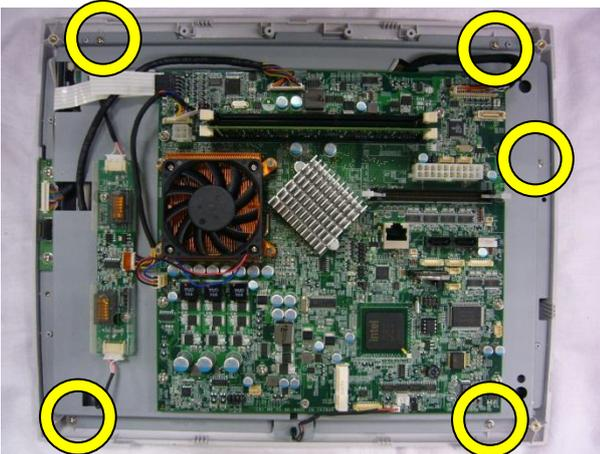
c. Remove the screws (5) that secure the LCD chassis. Then, remove the LCD chassis.
