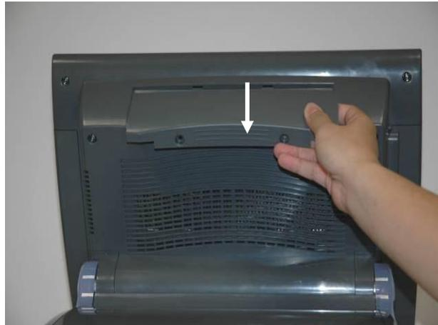
b. Slide the VFD dummy door out.
