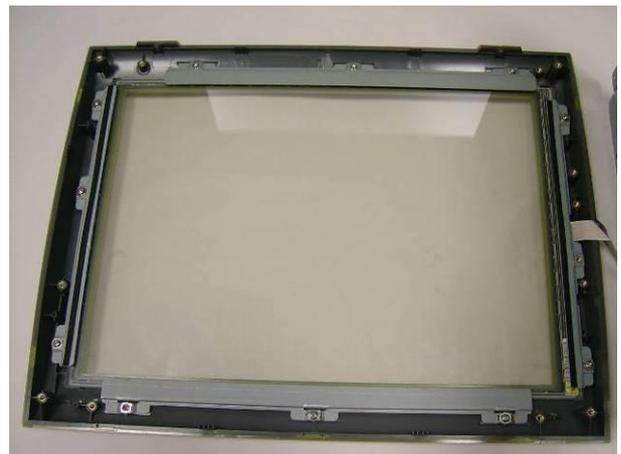
d. Remove the screws (12) to remove the touch panel.
