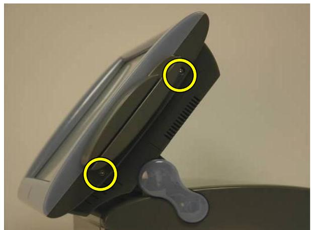
d. Fasten it to the display housing by tightening the screws (2).
