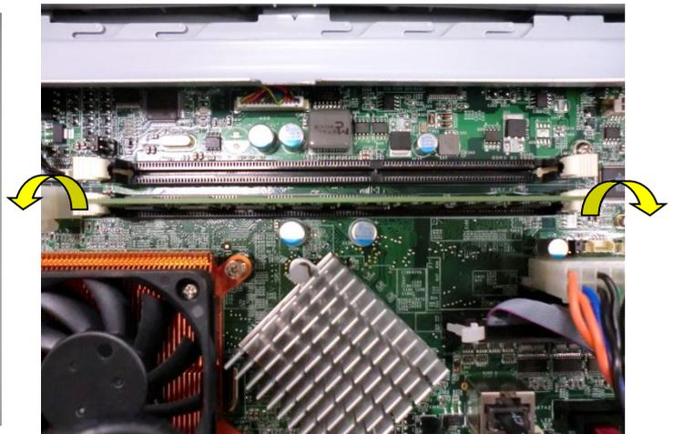
b. The memory slots are located on the mainboard. To remove the memory module, use your finger to push the DIMM slot ejector clips into the down position. Remove the memory module from the slot.
