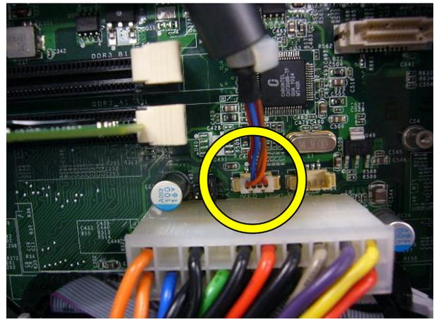
h. Connect the VFD cable to the connector as shown.
