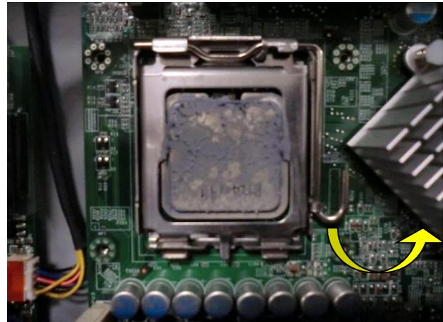
d. To remove the CPU, push the CPU socket lever down and away from the socket, and lift it up.
