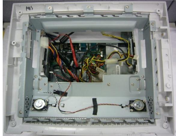
g. Then you will find the LCD chassis (left) and the base(right) separated as pictures shown. Remove all the remaining cables on motherboard.
