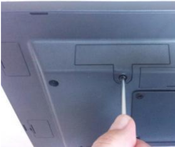
HDD access panel
