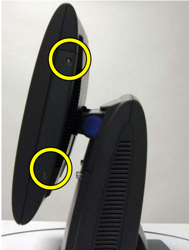
a. Remove the screws (2) to release the MSR dummy door from the system.
