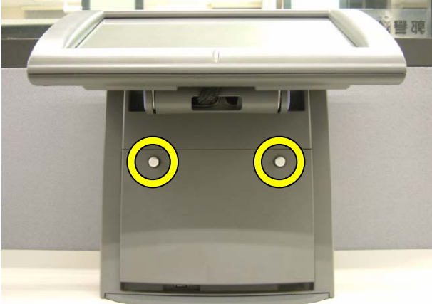
a. Loosen the thumb screws (2) to remove the front side stand cover.
