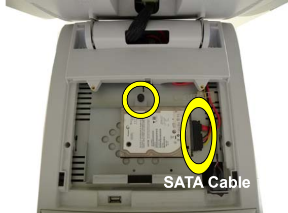
b. Disconnect the SATA cable (1) and loose the screw (1) to loose the HDD bracket from the system.
