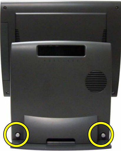
a. Loosen the thumb screws (2) to remove the front side stand cover.
