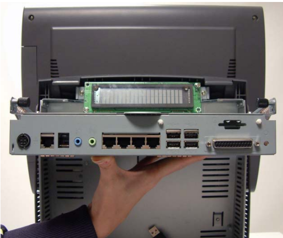
c. Lift the Main board module up to access to the I/O
