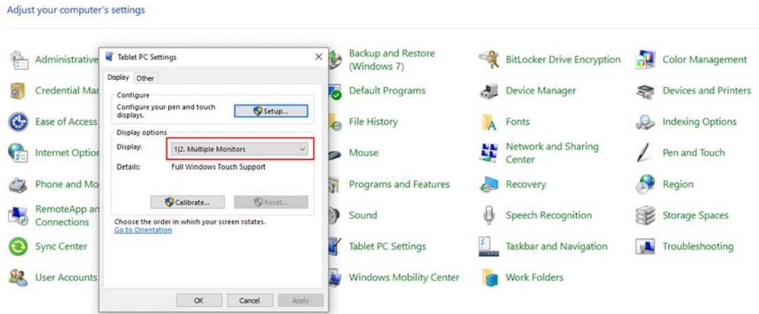
3. USC-360 main screen will show below picture, please touch main touch screen, then Press keyboard “Enter”; then on second display see same picture, if the second display has touch function, please touch it; if the second display no touch function, then Press keyboard “Enter”.
