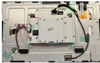
Install 1pcs Wi-Fi antennae on the wifi module
