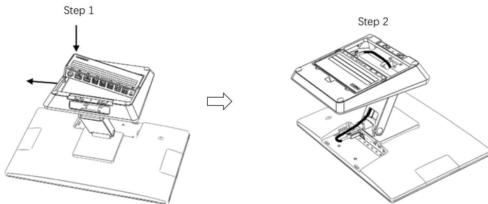
Firstly put one side of Hub into the slot of base, then push the other side of the Hub down as you pull the other side of the slot outwards with your hand.
