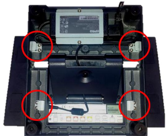
2. Next attach the mounting bracket to the wall or other surface using at least four of the bracket mounting holes. Please note that the bracket has both a 100mm and 75mm hole pattern, so that the bracket can be used with the VESA bracket as well as being directly mounted to a wall.
