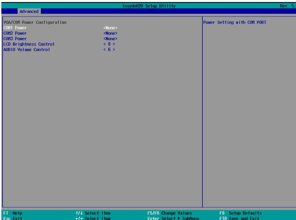
4. To enable the power, select COM1, COM2 or COM3 Power setting and press <Enter>. Select Power and press <Enter>. Save the change by pressing F10.
