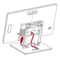
Step 1: how to remove the back cover.
