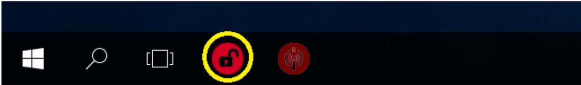
By clicking on the icon, the unlock program will run and unlock the Swing from the base. If the Swing is not removed within 5 seconds, the docking station will relock. If run when undocked the program does nothing.
