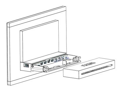
2. Remove the two side-screws to release the I/O Module.
